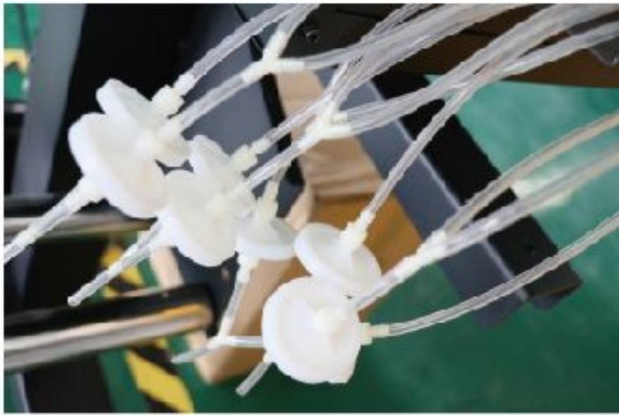
The automatic cleaning assembly adds a single-way valve to increase the stability of the ink supply
