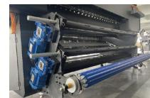
Air expansion shaft rubber strip rolls collection and release, to ensure that the collection of material more stable and flush
