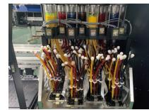
Negative pressure ink supply system: good for long time printing and cleaning
