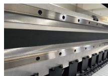
THK double guide rail is equipped with professional tooth-shaped belt transmission to provide silent and stable high-speed operation effect
