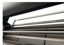
Swinging rod type feeding tension system
