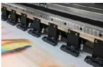
New independently adjustable three-stage pinch roller brings more stable feeding precision.
